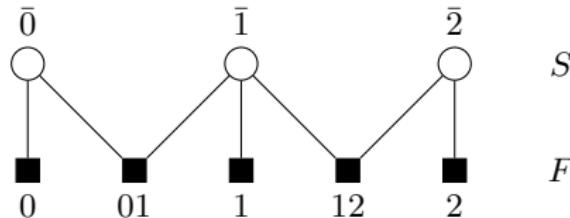
**Definition.** A triple  $(S, F, E)$  is called a **factor graph with variable nodes  $S$  and factor nodes  $F$**  iff  $S \cap F = \emptyset$  and  $(S \cup F, E)$  is a bipartite graph such that  $\forall e \in E \exists s \in S \exists f \in F: e = \{s, f\}$ .
